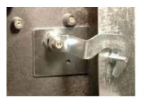
10. Close the door and test for a tight fit, bending the cam if necessary.
