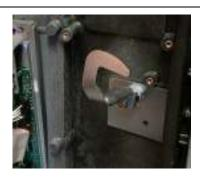
7. Close the door. Open the other door. Mark the spot below the arc of the cam as shown in the picture.
